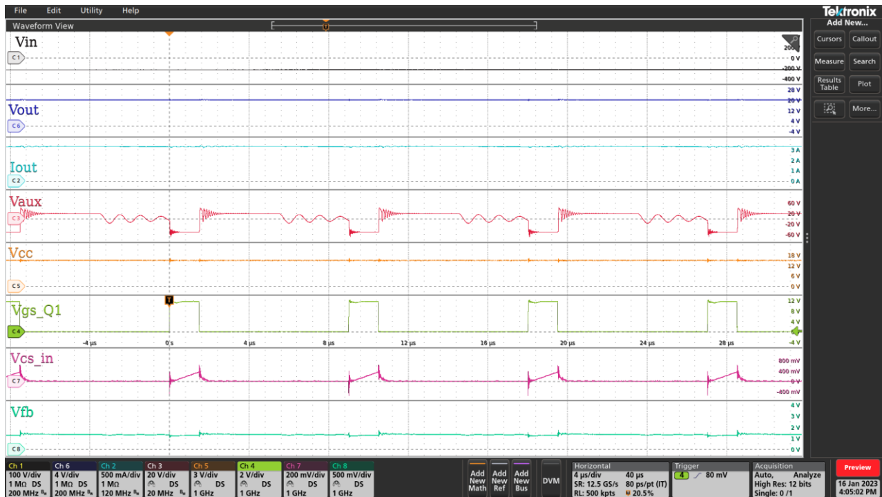
Figure 23 - The CGD quasi-resonant evaluation board waveforms at full load
