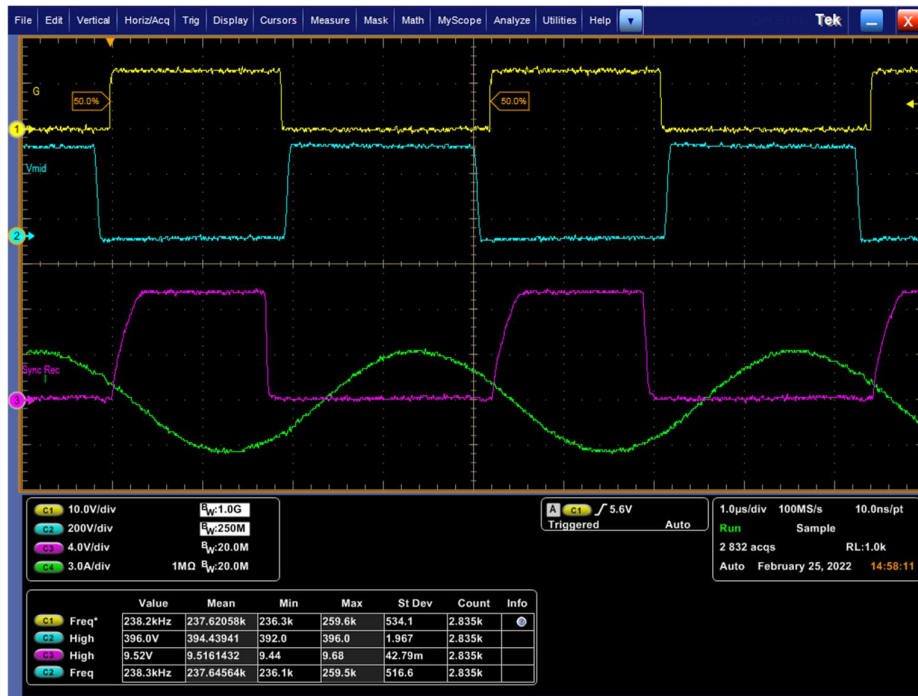
Figure 10 - LLC Eval Operating at 350 W. 2 \mu\text{s}/\text{div} .
