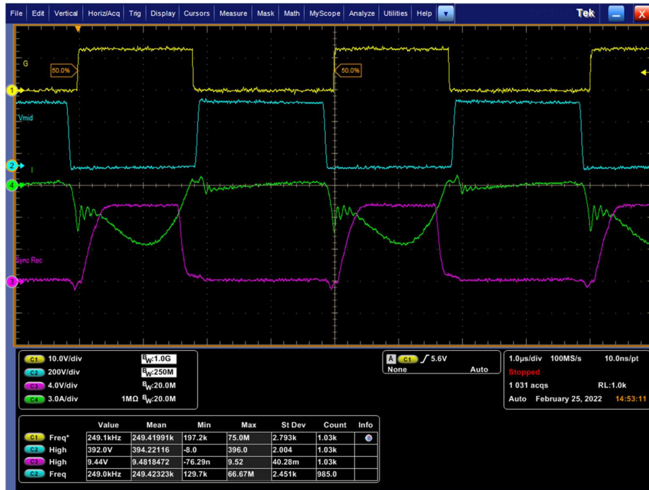
Figure 11 - LLC Eval Operating at 100 W. 1 \mu s/div.
