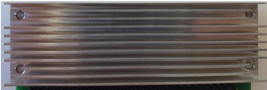
Figure 10 - Bottom-side cooling example: heatsink side
