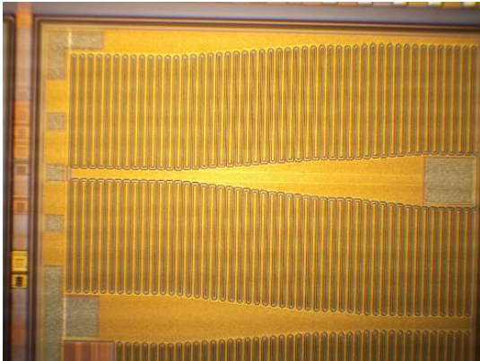
Figure 4 – ICeGaN™ Power HEMT featuring a smart interface and a tapered design of the source/drain metallisation for optimum current distribution.
