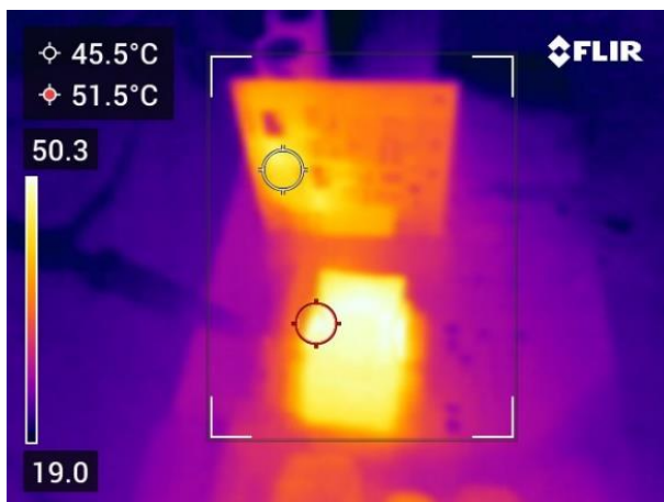
Figure 25 - Fast-leg high-side ICeGaN temperature after 40 min at 115 V AC / 350 W
